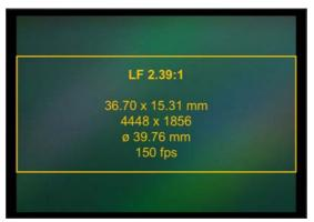
• Please note that the 2.39:1 sensor mode (4448 x 1856 pixels) has almost the same height as the ALEXA S35 3.2K sensor mode (3200 x 1800 pixels).
