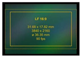
• Please note that the LF 16:9 sensor mode (3840 x 2160) has the same height as the ALEXA S35 6:5 sensor mode (2578 x 2160), which is used for shooting with anamorphic lenses.
